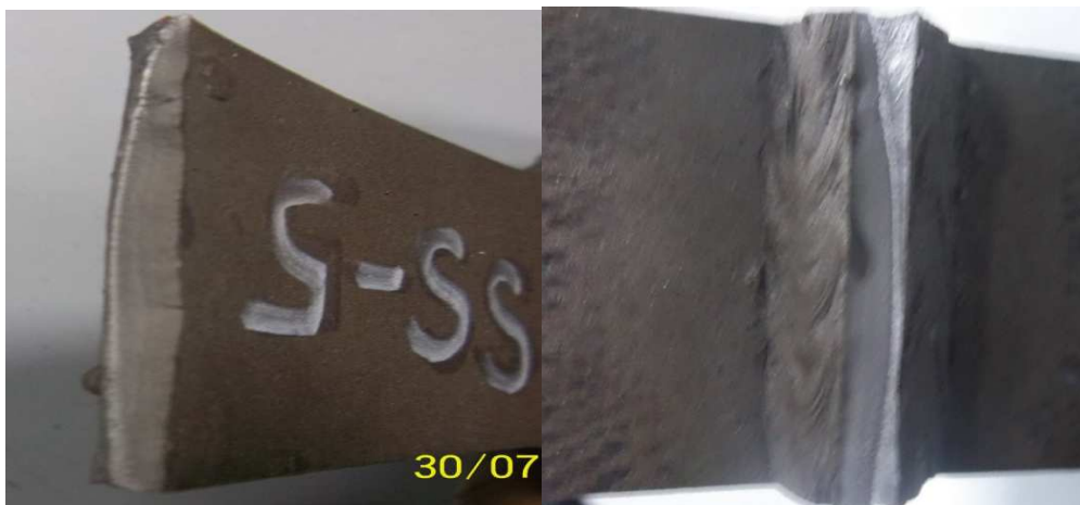
Figure 3. Fatigue failure showing crack propagation through weld toe
