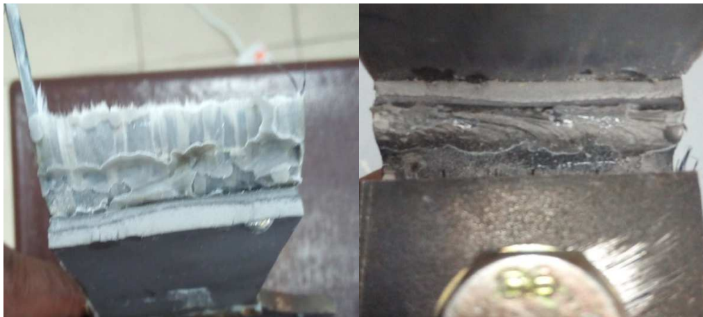
Figure 5. Failure of retrofitted specimen and bearing plate with bolts with no sign of debonding
