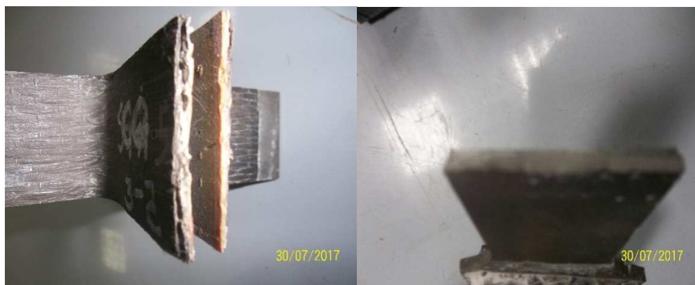
Figure 4. Failure of retrofitted specimen with FRP materials only with sign of debonding
